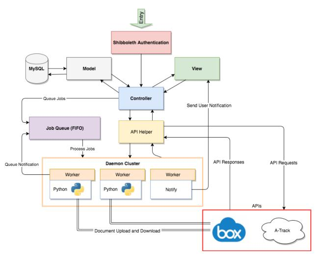
This diagram shows the Interaction between components of the web application.
